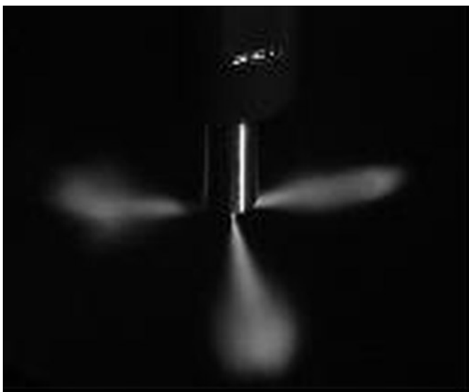
Fig. 6. Stream of the fuel injected in the injector with the catalytic coating applied
