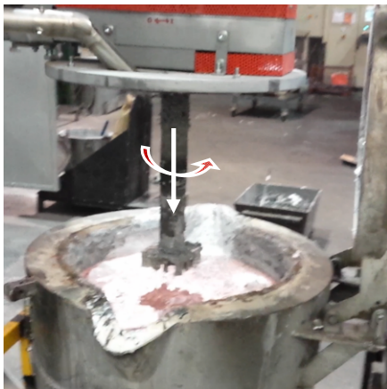
Fig. 4. Test stands used for testing: a) apparatus DTA-Cristaldigraph, DI-MK and FMA, b) rotor (refining process with argon)
