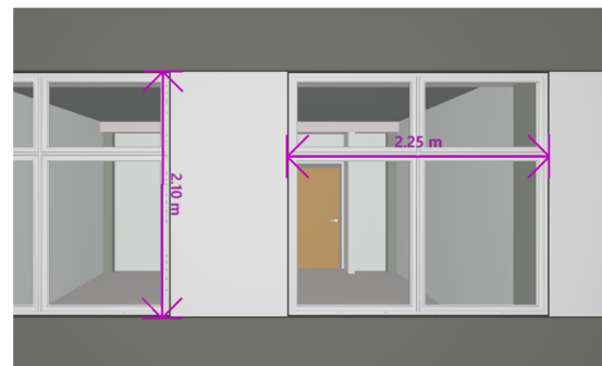
Fig. 8. Windows take-offs on the basis of the BIM model (source: own study)
