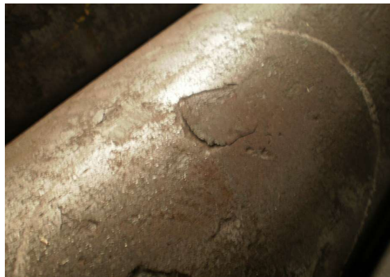
Fig. 3 The scale on the outer surface
