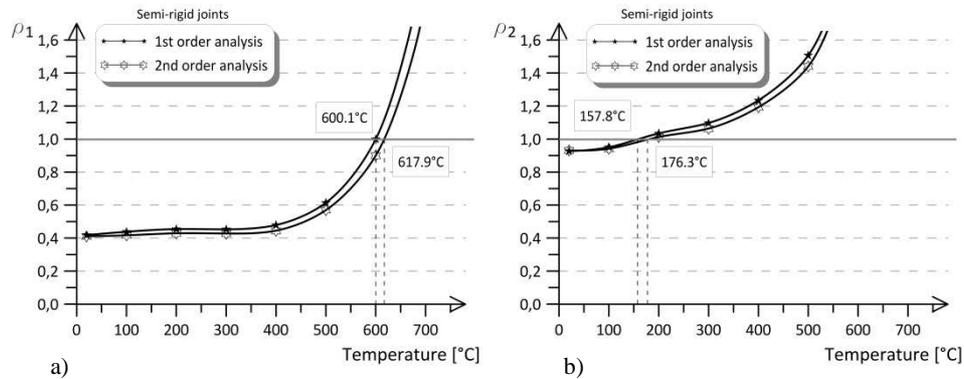
Fig. 10. Determination of critical temperature in the case of beam No 7, according to the first and second order theory, taking into account the joint stiffness changing with temperature, including: a) based on effort  $\rho_1$ , b) based on effort  $\rho_2$
