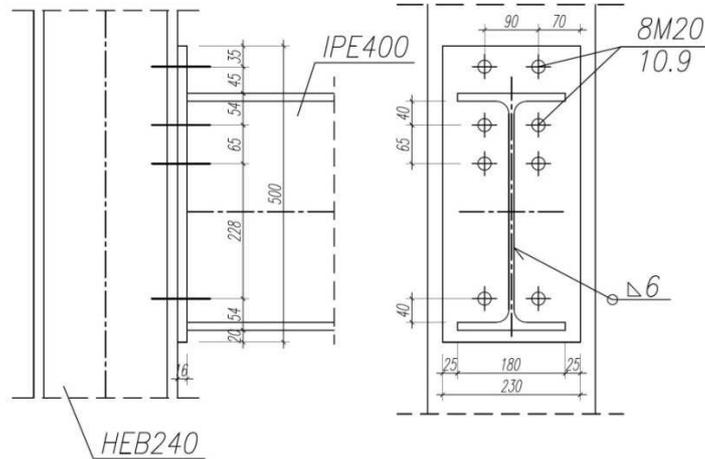
Fig. 2. Scheme of the beam to column joint used in the frame considered here
