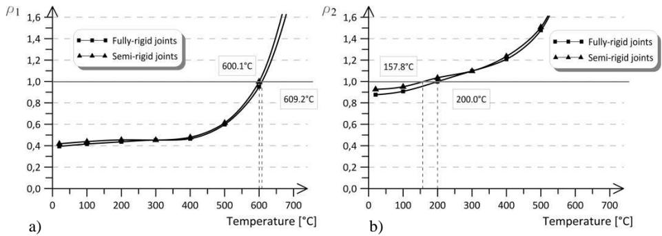
Fig. 8. Determination of critical temperature in the case of beam No 7, according to the first order theory, including: a) based on effort  $\rho_1$ , b) based on effort  $\rho_2$
