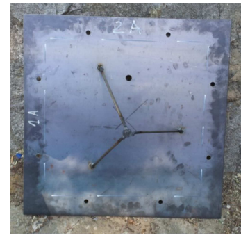
Fig. 5. Mounting base of internal pressure gauge
