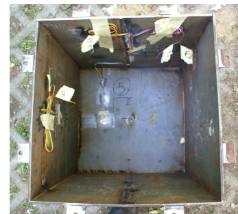
Fig. 6. Incident pressure wave gauge and strain gauges
