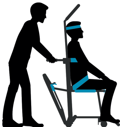
Figure 9. Evacuation chair with fixed four wheels (tilted backward) (EnSafe, 2023)
