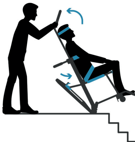
Figure 10. Method of tilting an evacuation chair with fixed four wheels (EnSafe, 2023)
