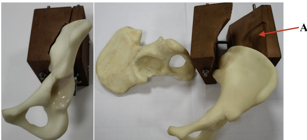
Fig. 5. The fixture design for pelvis model
