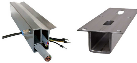
Fig. 1. Multifunctional sheet metal profiles produced by the CRC 666 production line
