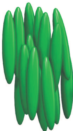
Figure 2. Nematic phase represented schematically
