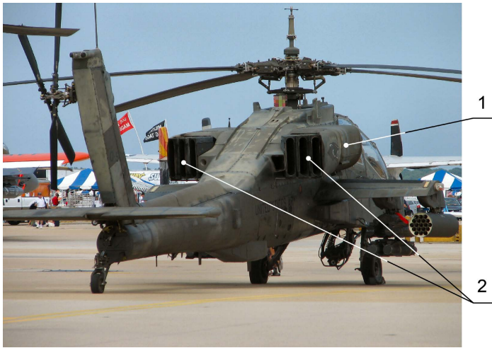
Fig. 23. AH-64 Apache rear view, 1 – engine, 2 – exhaust cooler, [21]
