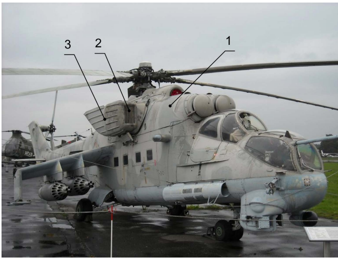
Fig. 24. Mi-24 Hind helicopter after modernization, 1 – engine, 2 – exhaust cooler air intake, 3 – exhaust cooler, [21]
