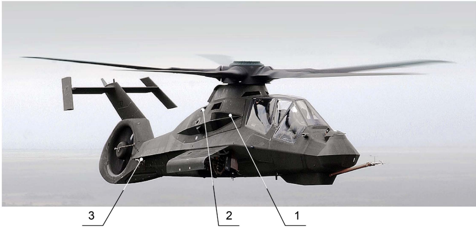
Fig. 25. RAH-66 Comanche prototype in flight: 1 – engine air intake, 2 – exhaust cooler air intake, 3 – exhaust system, [21]
