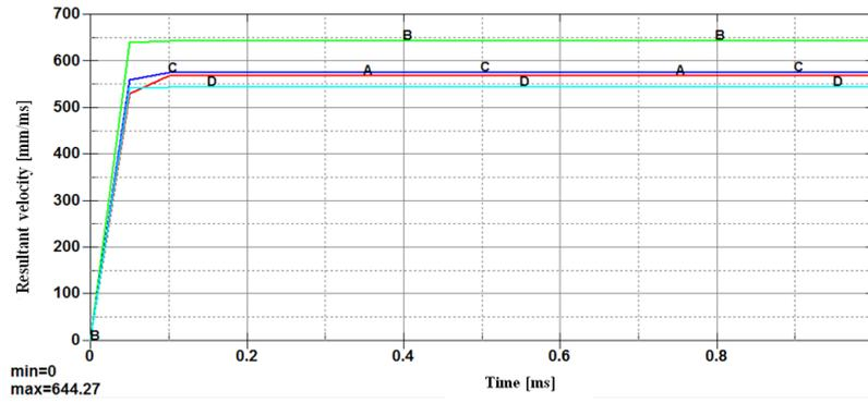
Fig. 9. Time-velocity graph for fragments originating from detonation point – top layer
