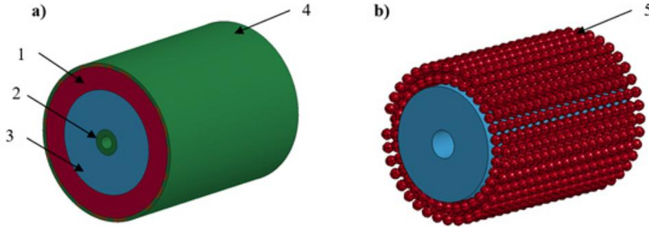
Fig. 2. Numerical model of the cylindrical fragmentation warhead a) entire model b) fragmentation liner, 1 - fragmentation liner, 2 - inner case (optional), 3 - explosive charge, 4 - outer case, 5 - steel balls
