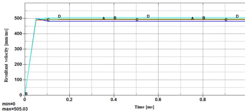
Fig. 12. Time-velocity graph for fragments originating from detonation point – top layer
