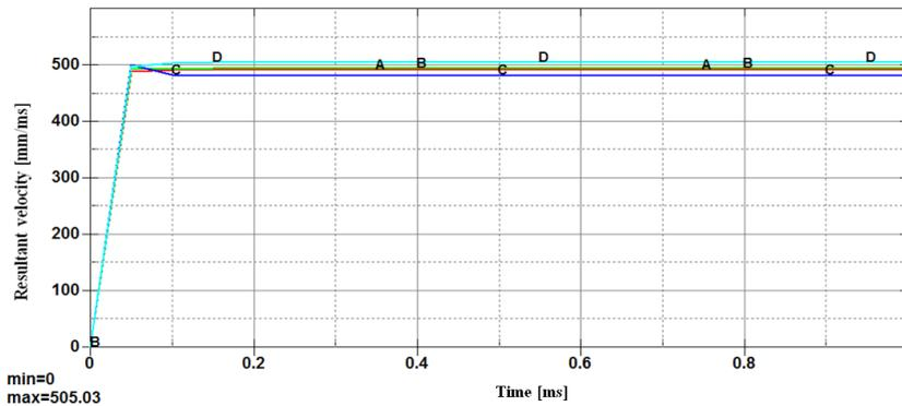
Fig. 11. Time-velocity graph for fragments originating from right end – top layer
