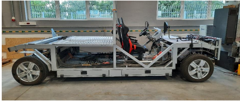
Figure 5. A man-driven prototype platform equipped with the in-wheel DWH-200 motor. Source: Arex
