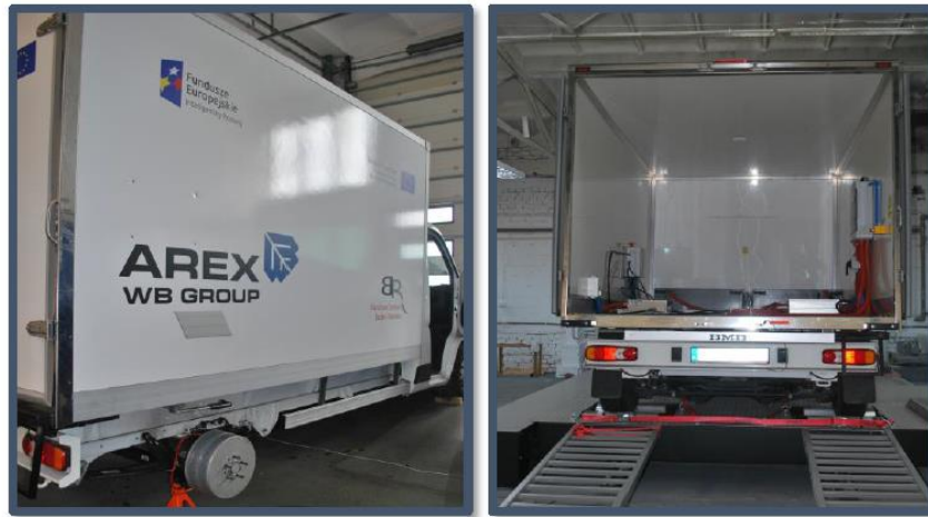
Figure 6. DWH-200 motor mounted as a rear-drive configuration of the Peugeot Boxer. Source: Arex.
