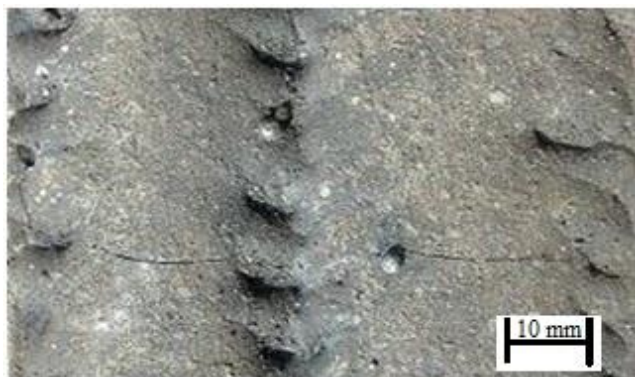
Fig. 16. Face inequalities by automatic welding.
