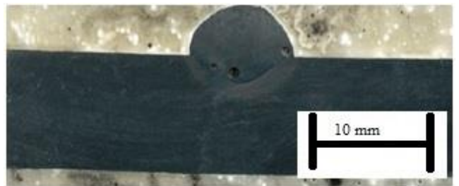
Fig. 8. Gas pore in the single layer of the weld
