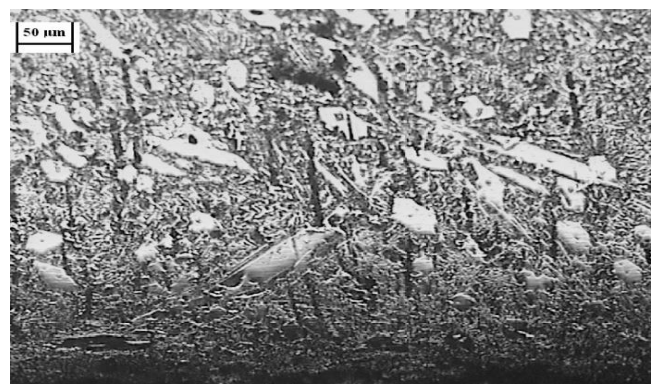
Fig. 3. Structure of material over the fusion line
