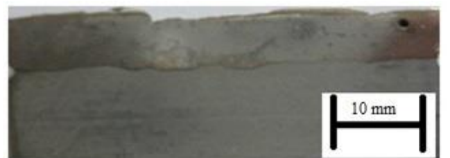
Fig. 9. Gas pore in the wide layer the weld
