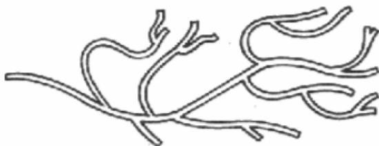
Fig. 4. The structure of low-density polyethylene (LDPE) macromolecules [L. 19]
