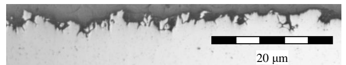
Fig. 8. Microstructure the X55CrMo14 steel after 144 hours soaking in 65% nitrate acid at 348 K
