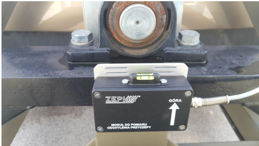
Fig. 4. Method of mounting the measuring module
