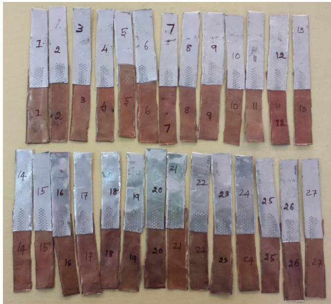
Fig. 4. Al-Cu Welded samples
