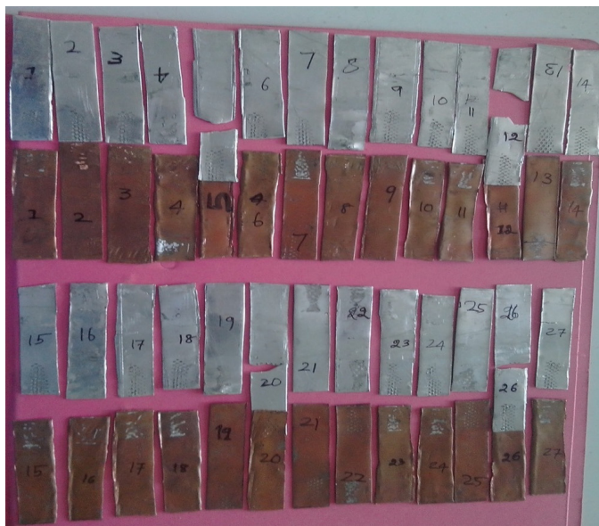
Fig. 5. Tensile strength tested specimen
