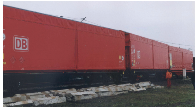
Fig. 20. Two-axle wagon with sliding walls tested in the additional variant in which the wagon is surrounded by two identical wagons [photo. A. Zbieć]
