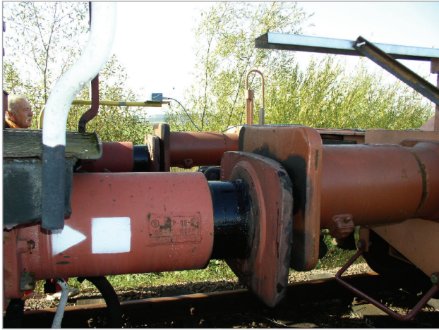
Fig. 6. 80 mm difference in the height between the buffer centre lines of the test wagon and barrier wagon [photo. A. Zbieć]
