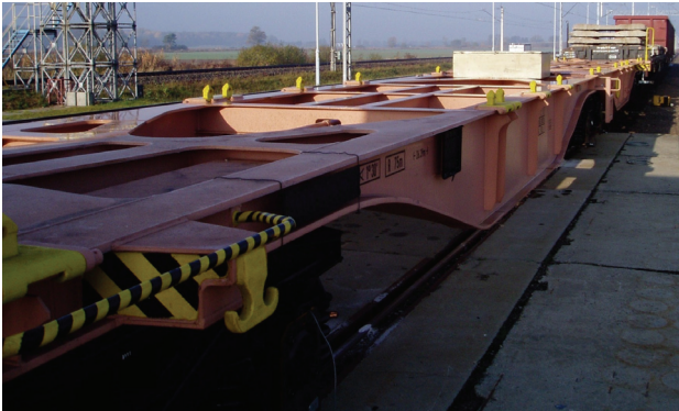
Fig. 22. Two-section platform wagon on three bogies – two leading bogies and one middle bogie [photo. A. Zbieć]
