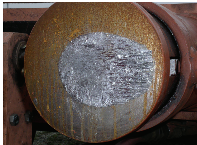
Fig. 8. Grooves and burrs on the surface of a diagonal buffer [photo. A. Zbieć]
