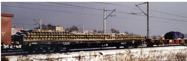
Fig. 16. Two-axle platform of the length 17.4 m and long overhang 3.7 m [photo. A. Zbieć]
