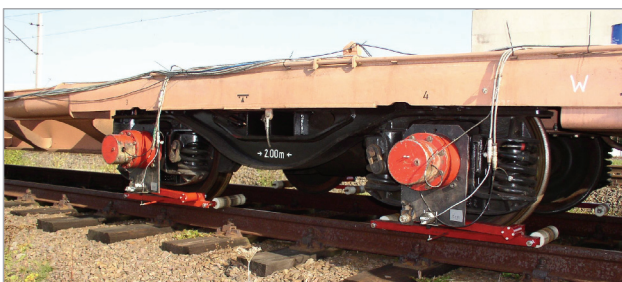
Fig. 7. Heads for measuring lateral forces and equipment for measuring wheel uplift [photo. A. Zbieć]
