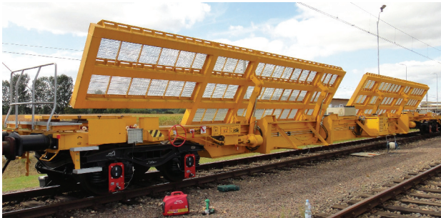
Fig. 23. Two bogie 27.5-metre-long platform for railway switch transportation [photo. A. Zbieć]
