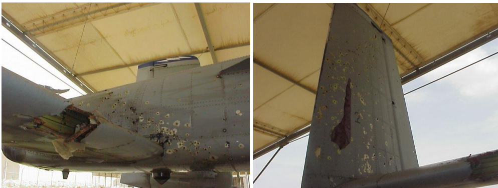
Fig. 1. Battle damages of A-10 aircraft during 'IRAQI FREEDOM' operation. Source: Own study based on [2951st Combat...].
