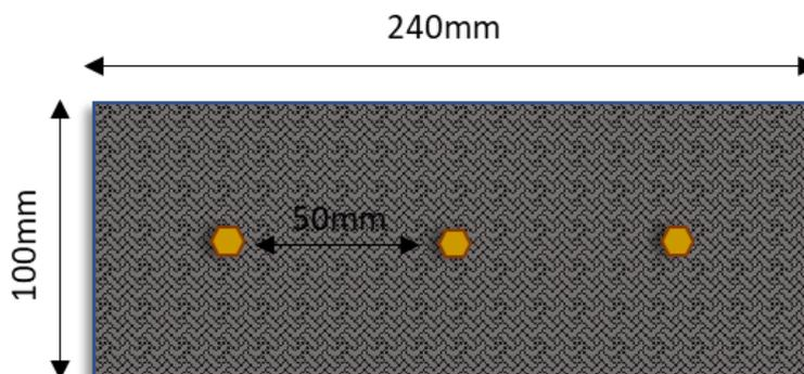
*Fig. 2. Three-screw sample dimensions*
