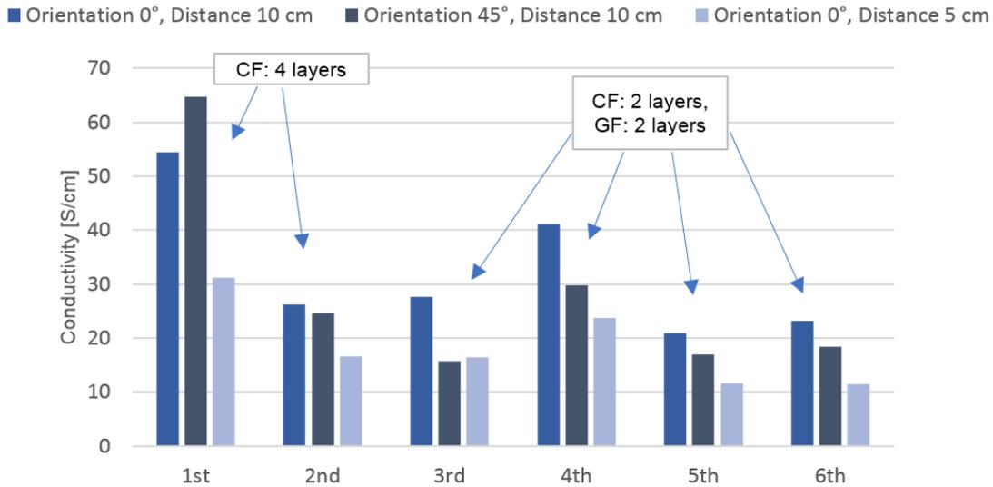
Fig. 3. Electrical conductivity of all samples, I (0°) and II (45°) orientation
