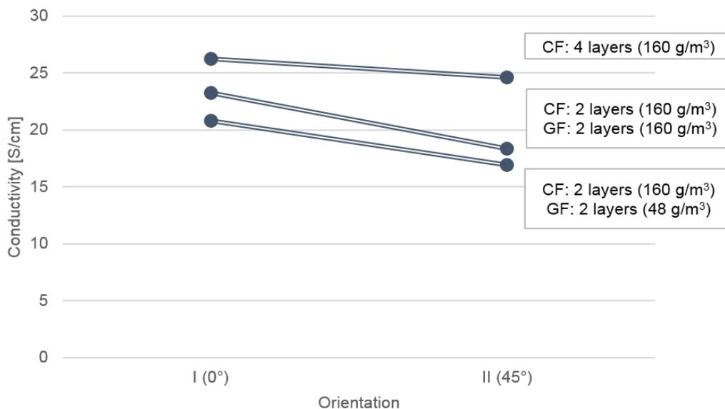
Fig. 6. Electrical conductivity depending on the fibre orientation, CF density of 160 g/m<sup>3</sup>
