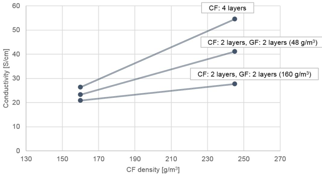
Fig. 5. Electrical conductivity as a function of CF reinforcement density, I orientation (0°)
