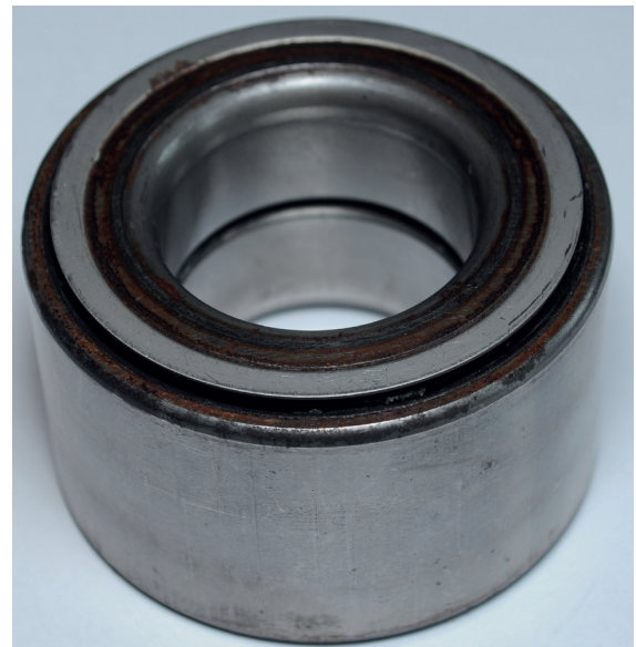
Fig. 4. Bearing VKBA 6831 from wheel of Toyota Avensis
