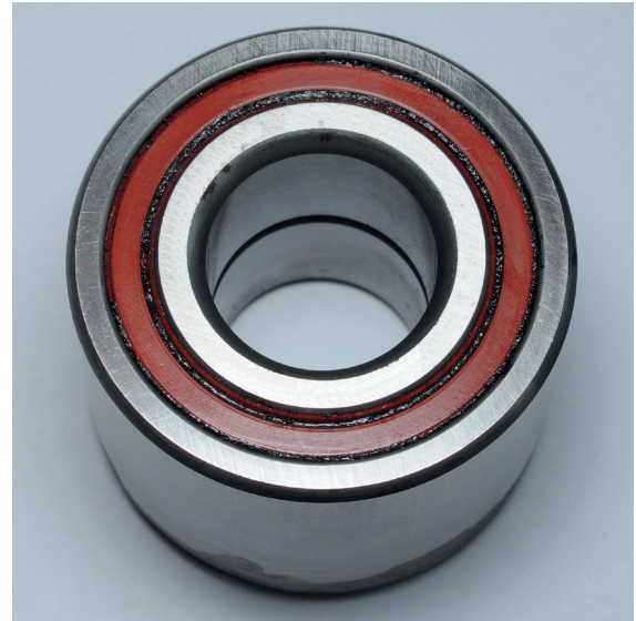
Fig. 3. Bearing VKBA 3692 from wheel of Renault Kangoo
