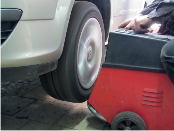
Fig. 5. Wheel balancer used to speed up wheels
