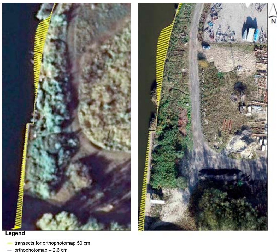
Figure 7. Transects between the sonar image and the orthoimage of 2.6 cm (left) and 50 cm (right)
