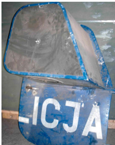
Fig. 3. Right-hand door of the Mi-2 helicopter enabling aerial images to be taken in a vertical position. Walenty Tieśluk's file.
