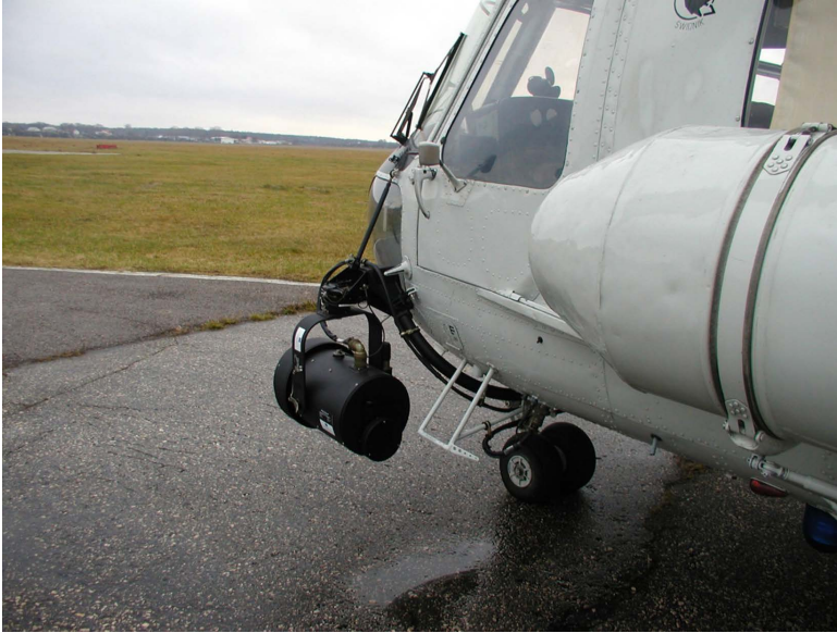
Fig. 7. SX-16 floodlight mounted on the Mi-2 helicopter. From the author’s file.
