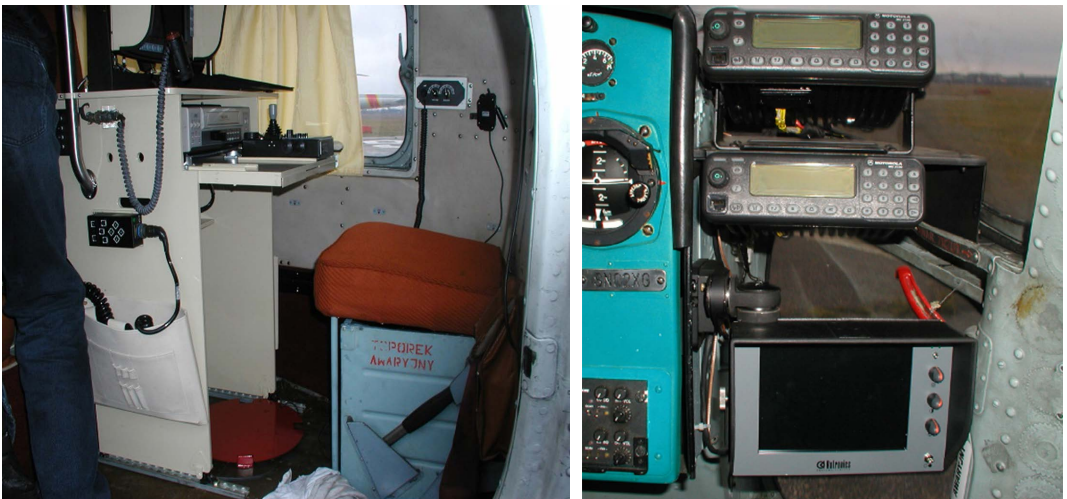
Fig. 8. left – station of the UltraForce 275 in-flight observation system operator; right – system’s monitor used by the pilot, located under on-board radios. From the author’s file.
