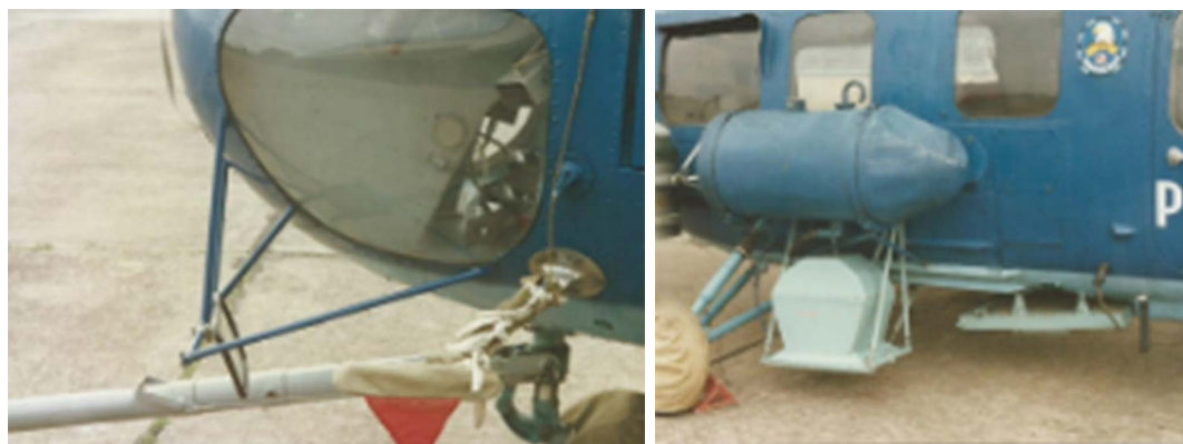
Fig. 5b. Special equipment: left – pilot’s mirror; right – speaker and grenade launcher under the airframe. Marek Dominiak’s file.
