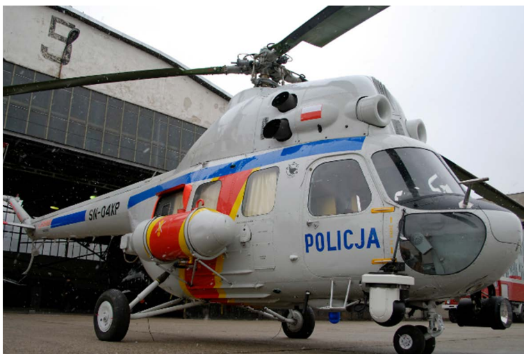
Fig. 11. Mi-2 helicopter handed over by the Border Guard to the Police. Instead of being removed, the Border Guard livery was only covered with the Police livery. Image: Paweł Kłosiński.
