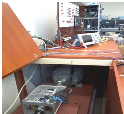
Fig. 13. General view of the measurement set used for the investigation of the 5.5 kVA salient pole synchronous generator with the three rotor structures
