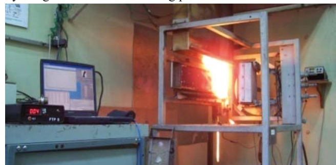
Fig. 1. Research rig examining surface flammability level of materials according to FTP Code, part 5
