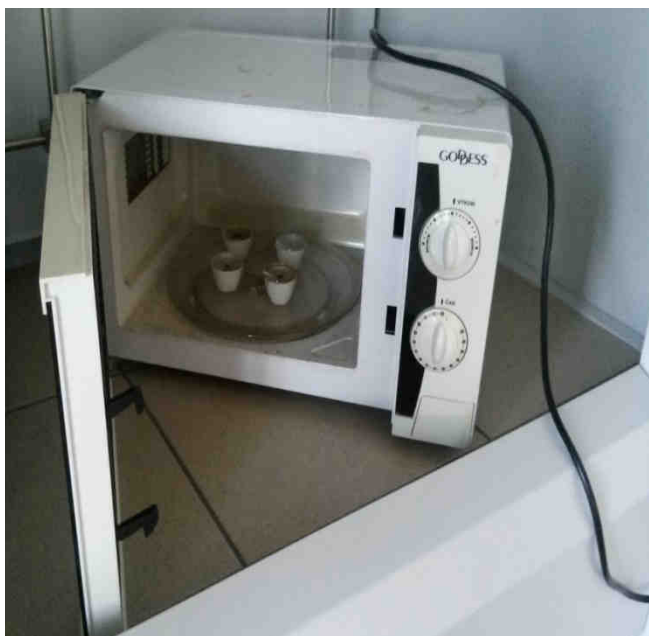
Fig. 6. Kitchen microwave oven with four crucibles containing reaction mixtures of formic acid and four different aniline derivatives
