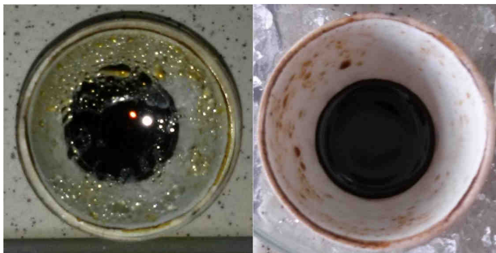
Fig. 8. Crucible with the product of the reaction of formic acid with 4-methoxyaniline
