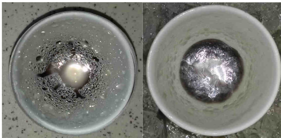
Fig. 9. Crucible with the product of the reaction of formic acid with 4-chloroaniline
