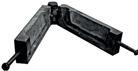
Fig. 3. Metal (cast iron) mold for casting bars for strength test
