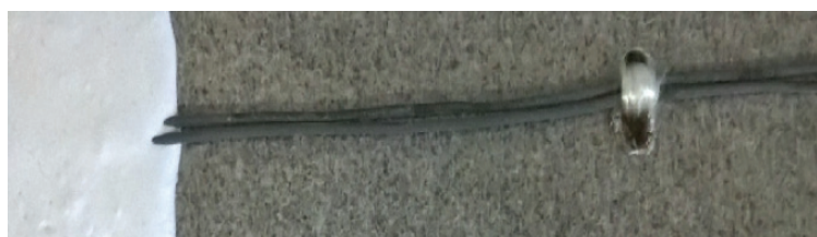
Fig. 8. Small part of the 3m length bifilar line set on a mica plate
