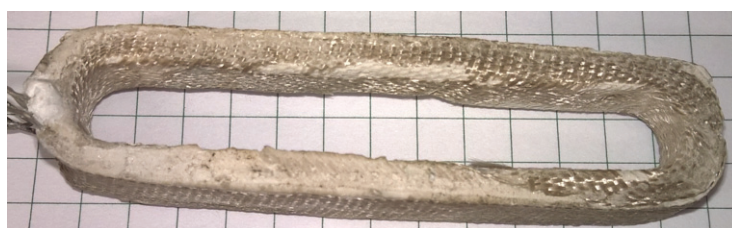
Fig. 1. HT° inorganic coil after tests at 500°C
