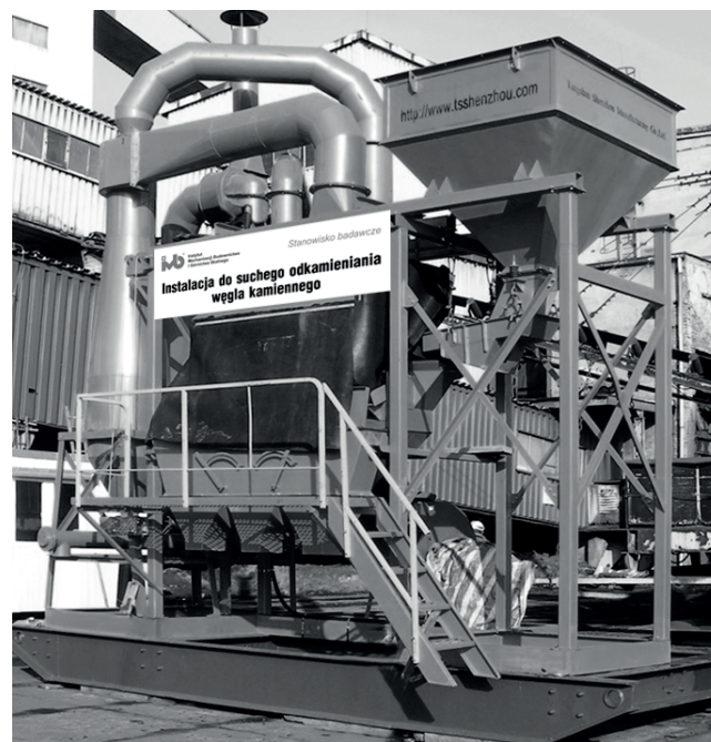
Pic. 1 Air concentrating table of FGX – 1 type
