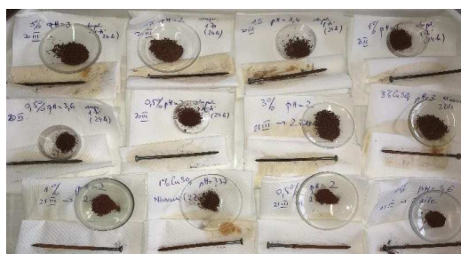
Fig. 3. Samples with the amount of copper deposited on the iron, from different days of the experiment
