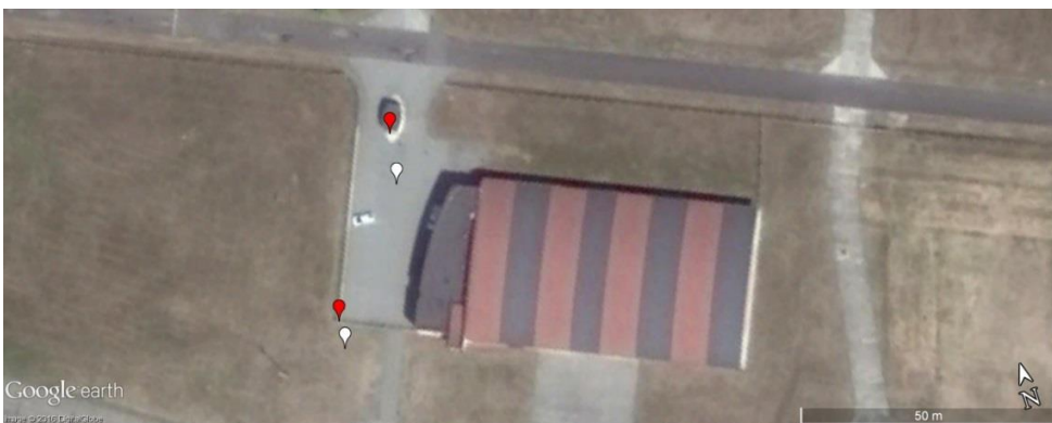
Fig. 8. Results of the georeference (red markers – Google Earth, white markers – SAR) [used application Google Earth]
