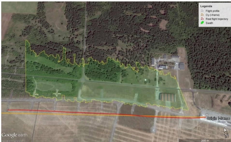
Fig. 5. UAV real and theoretical flight trajectory [used application Google Earth]
