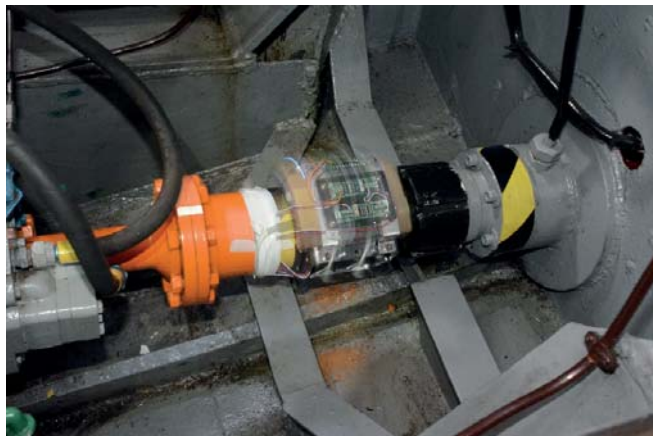
Fig.3. Torque and thrust measurement system rotating with the propeller shaft during the measurements
