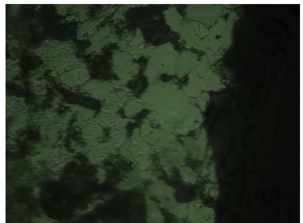
Fig. 14 Microstructure of steel S355 J2G3 after AWJ cutting 600x
