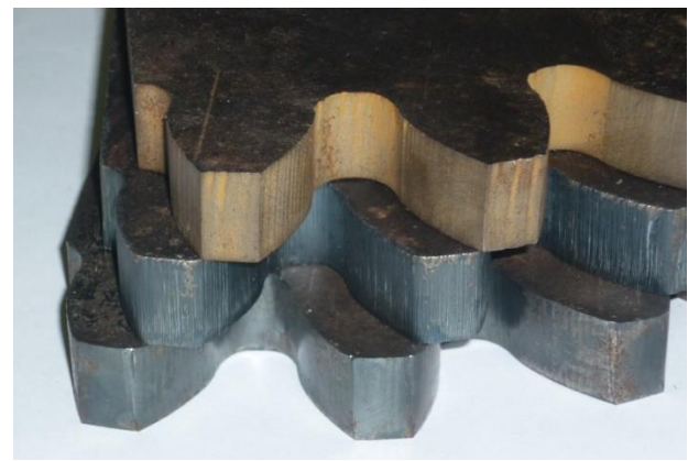
Fig. 5 Samples of tothing manufactured by cutting in ascending order – AWJ, laser, plasma
