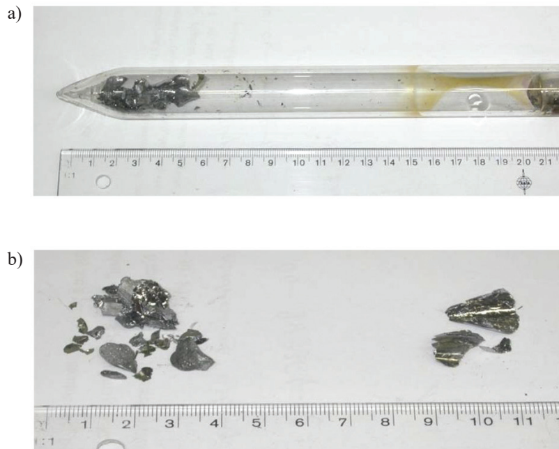
Fig. 8. Preparation of BiTeI semiconductor in BTI C2 process by CVT method in a horizontal configuration: a) view of the reaction ampoule, b) the reactants of the precursor (left side) and the deposited BiTeI layers (right side).
