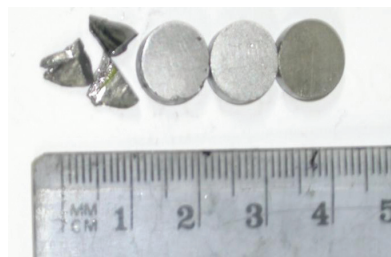
Fig. 17. BTI-2 crystal after cutting it into wafers of a thickness of approx. 4 mm, destined for the structural and electrical measurements.
