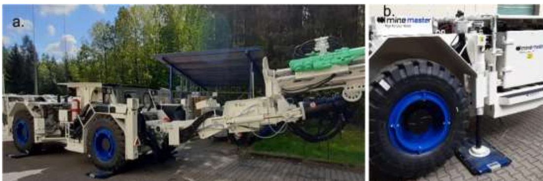
Fig. 10 Measurements of the pressure force of Roof Master 1.7 K wheels and supports on the ground – model validation
