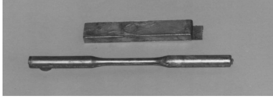
Fig. 2. Composite castings for mechanical and tribological investigations
