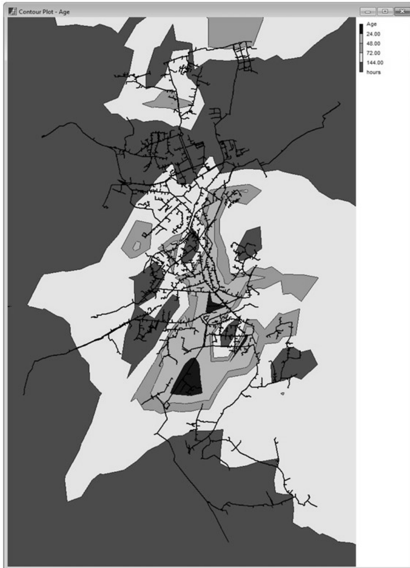
Figure 8. Age of water in WDN Polanica-Zdrój – simulation time 240h. Variant 1
