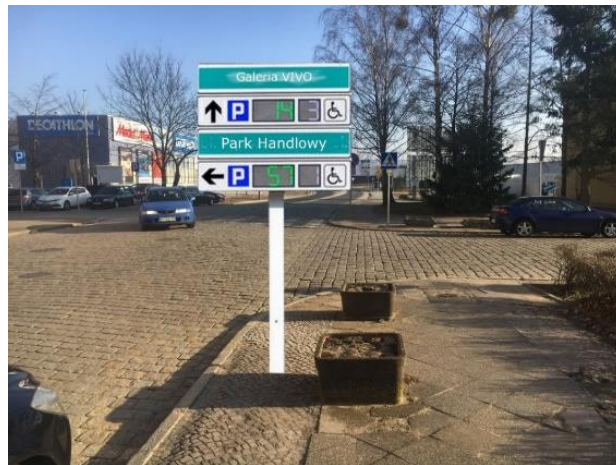
Fig. 3. Visualisation of the variable content sign indicating the number of free parking spaces - the sign is located on Staszica Square Source: authors' study based on [17]
