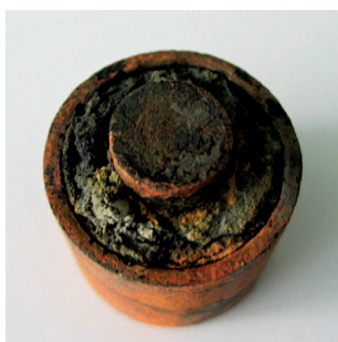
Fig. 1. Sample of set cement not resistant to H 2 S, deposited in formation water saturated with hydrogen sulfide (compressive strength 1.5–2.0 MPa)
