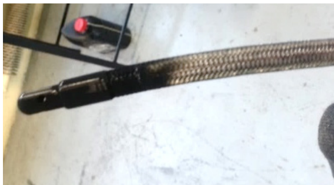
Rys. 10. Zadymiona sonda analizatora spalin Bosch BEA 250 (fot. S. Kilimnik) Fig. 10. Smoked probe of exhaust gas analyzer Bosch BEA 250 (photo by S. Kilimnik)
