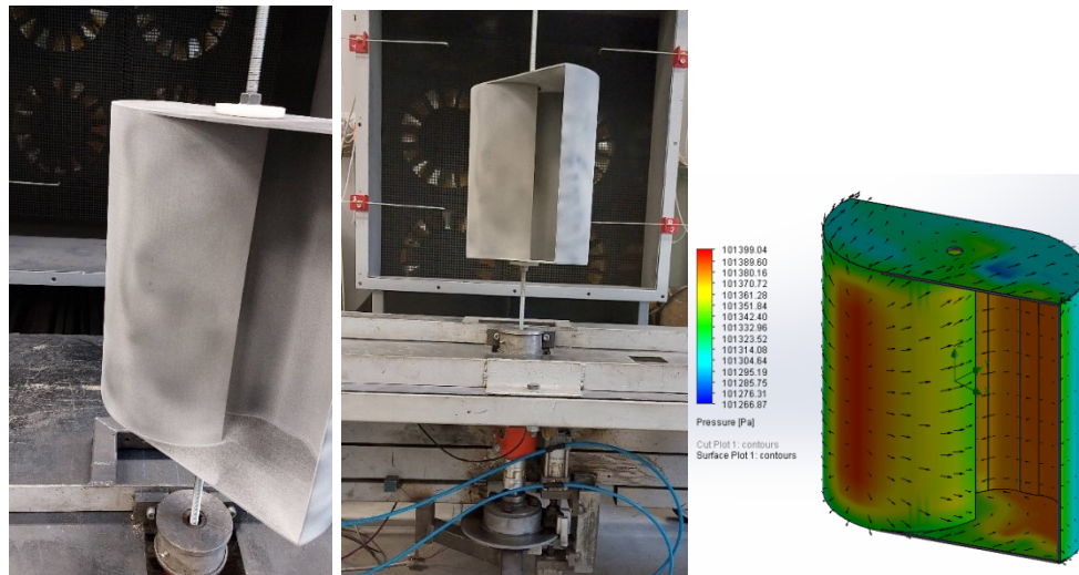
Figure 7. View of the printed model on the test stand and isometric view of the pressure distribution on the blades of wind turbines at a wind speed of 10 \text{ m}\cdot\text{s}^{-1} .
