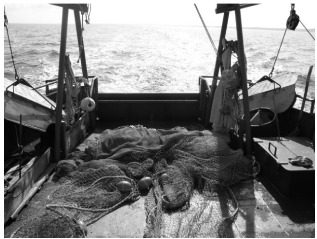
Phot. 4. Gate-like gallow construction of trawl blocks
