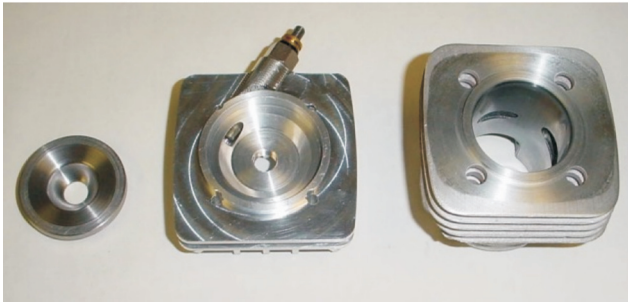
Fig. 8. SCS two-stroke HFE system components: combustion chamber insert (left), cylinder head with glow plug heater (middle), original factory made cylinder body (right) [7]
