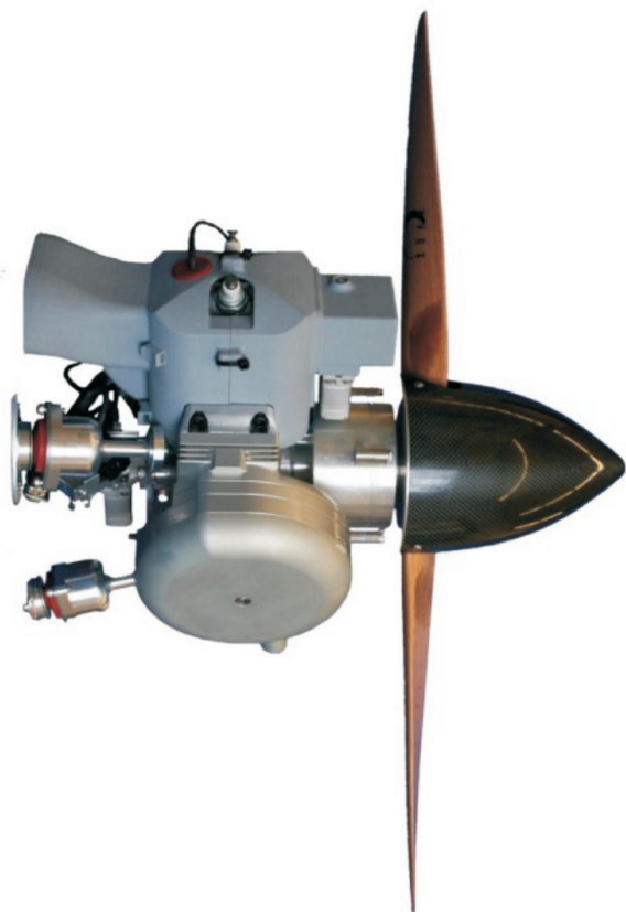
Fig. 21. NW-44 EFI HFE engine; basic configuration [27]
