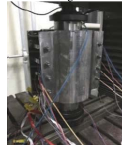
Fig. 17. Long bolt form grouting clamp and strain gauge on the side of bolt
