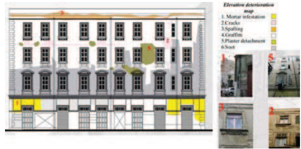
Fig. 17. Different types of deterioration on Wekalet El-Lamoun residential façade
