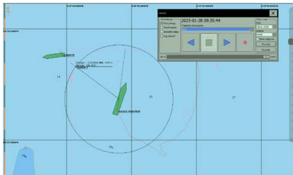
Figure 2. Distance between SHIP 1 and DIVER 2 diving boat = 0,24 NM = 449 m. Source: VTS Gdansk [5].
