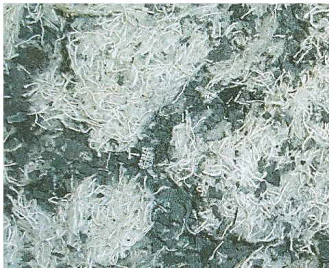
Fig. 3. 'Lamin' fabric granulate: volumetric density: 40 \text{ kg/m}^3 , cotton fibres shaken to obtain wadding form, slightly contaminated with rubber granulate, grain size: 2 \times 2 \text{ mm}
