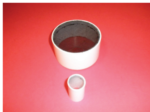
Fig. 5. Sleeves, 30 and 100 mm in diameter, to examine 50 mm-thick material layer
