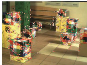
Fig. 7. a) Feature points selected for rotation angle estimation, b) Disparity vectors of feature points after image rectification.
