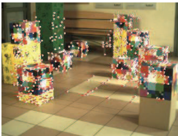
Fig. 6. Examples of 3D scene images with feature points and their disparity vectors without proper image rectification.
