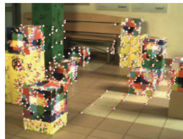
Fig. 6. Examples of 3D scene images with feature points and their disparity vectors without proper image rectification.
