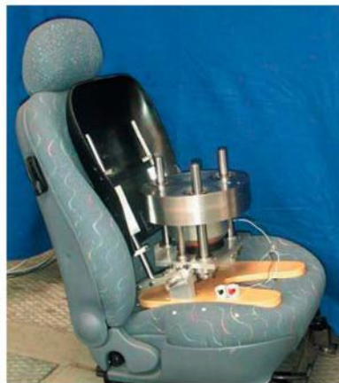
Fig. 6. Anthropodynamic dummy MEMOSIK IV placed on a motor vehicle seat [13]
